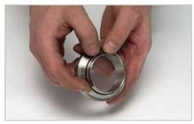
Fit the insert cone into the tube flare. If needed, tap gently with plastic or hide mallet.
