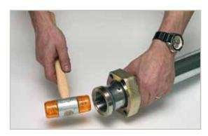
Lubricate the bonded seal (dowty seal) with Gleitmo 805 -paste or equivalent.
