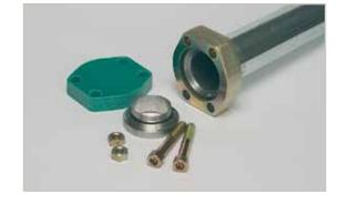
Lubricate the O-ring with Gleitmo 750 or equivalent lubricant. Place O-ring carefully into its groove. Examine all sealing surfaces to detect possible rust or mechanical damages.
