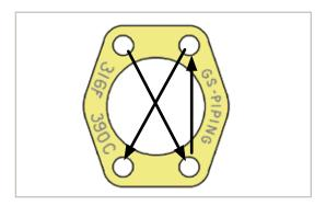
Tighten bolts in diagonal sequence in small increments to appropriate torque level. See illustrated example.
