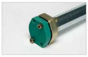
After the flare is checked and cleaned the pipe end is covered with a plug or tape.
