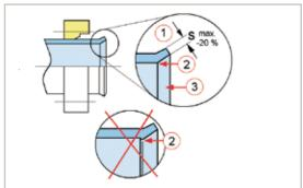
The thinning of the flared part of the tube "S" may not exceed 20% of wall thickness (1).
