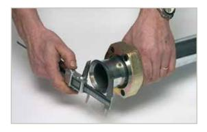
Verify the outside dimension of the flaring (Appendix 1, page 13) and check that the flare is concentric with the pipe.
