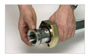
Check all seals and sealing surfaces of components and ensure that there is no damage.
