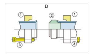
With an extra sleeve there is a possibility to have flange and pipe with different nominal sizes (i.e.  $38 \times 4$  pipe can be used with  $1 \cdot 1/4$ " SAE flange).
