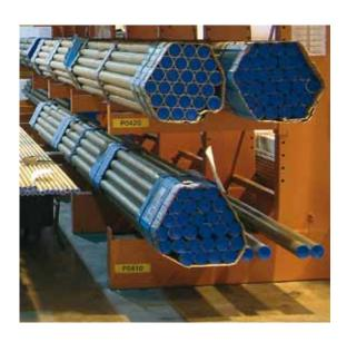
Always keep the pipes stored indoors away from rain and moisture. Make sure all the pipes are protected with plastic plugs in the ends.
