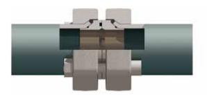
The GS-37° Flare System is used for piping with pressure with ranges of 50–420 bar. Extensive test programs – including rigorous vibration testing – have proven the suitability of the GS-37° flare flange system for a wide range of different materials and applications. GS-Hydro solutions are approved by many Classification companies for a wide range of materials and applications.
