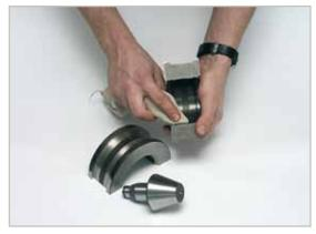
Clean the flaring cone and dies before fitting to the flaring machine. Also ensure the correct size cone and dies are selected for the pipe size.
