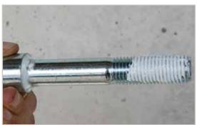
Inspect the bolts and nuts to ensure no damage. Lubricate bolt threads amply according to illustration. Spread evenly with a brush.
